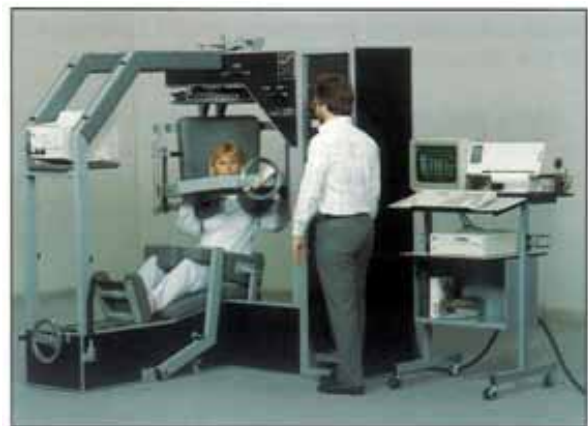
FIGURE 1-17 Both testing and exercise for the totally isolated muscles that rotate the torso are conducted in this machine; but since movement occurs in a lateral plane there is no need to counterweight the subject, torso-mass torque is not a factor. The muscles that rotate the torso are second in importance only to the muscles that extend the lumbar spine.
