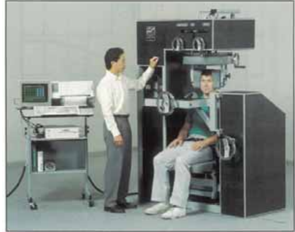
FIGURE 6-15 Because of the greater range of movement, with normal subjects, tests are conducted in a total of eleven positions, in increments of 12 degrees; but with a limited-range subject, tests can be conducted in increments of 6 degrees if desired.
