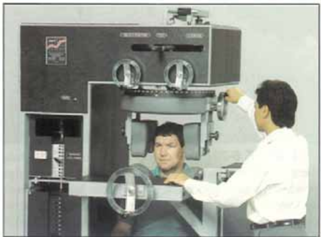
FIGURE 6-20 Turning this crank tightens the head-restraint pads.
