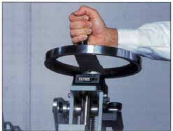
FIGURE 1-7 With subject relaxed in the extended position, the counterweight is adjusted by turning this crank until balance is provided; when properly adjusted, the weight of the body parts is balanced by the torque from the counterweight acting in an opposite direction. Proper counterweighting is clearly established by the computer monitor, which will tell you when the subject is balanced.
