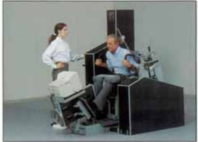
FIGURE 1-9 With the subject relaxed in the forward position, the computer monitor will show a bar-graph of torque; moving into this position compresses tissue in the front and stretches tissue in the rear of the torso, and this stored energy will produce torque in the direction of extension of the spine.
