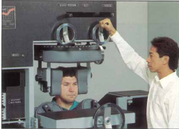
FIGURE 6-21 Seated and properly restrained, in a neutral (straight-forward) position, movement of the head is prevented by the range-limiting system. Initial prevention of movement is required as a first step in the measurement of cervical-rotation range of movement on an individual basis.
