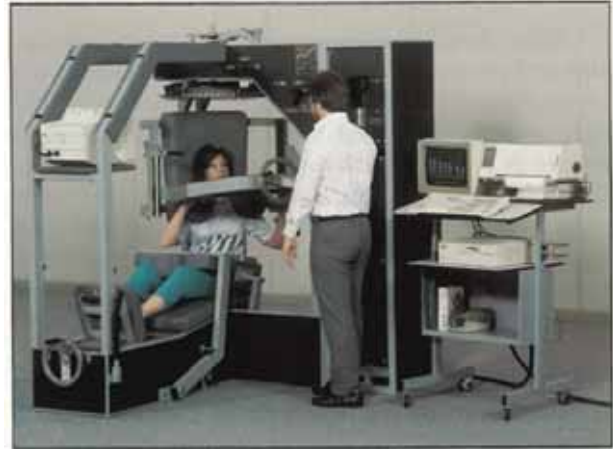
FIGURE 6-9 The pelvic-restraint system used for torso-rotational testing is similar to the system used in the lumbar-extension machine; but is designed to prevent pelvic rotation around a longitudinal axis, rather than in the direction of extension. When the torso is rotated, the pelvis will rotate together with the spine if such movement is possible, and this pelvic movement makes it impossible to measure true spinal rotation; so the pelvis must be restrained, and can be.
