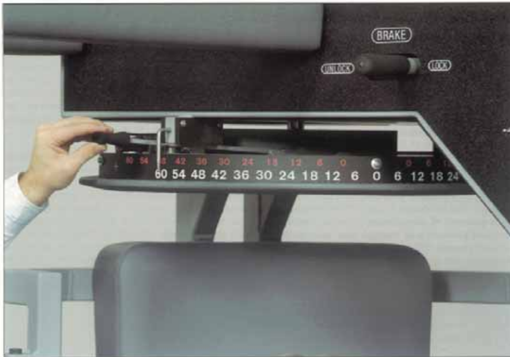
Figure 6-10 A locking system located above the subject limits movement to any desired range, in increments of 6 degrees. Thus locked, it is then impossible for the subject to move past the end of the selected range.
