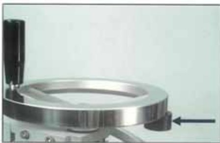
FIGURE 6-26 The wheel located on top of the counterweight for head mass is used for adjustment of counterweight torque, and the weight of the black handle used for adjustments is individually counterweighted by the small weight located directly opposite the handle position; providing a perfect degree of counterweighting even for parts with a weight of only a few ounces.
