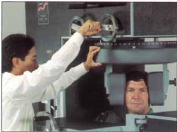
FIGURE 6-22 The subject is instructed to rotate their head, first in one direction and later in the opposite direction, producing a very low level of effort; and while the subject tries to turn the head, the therapist turns one of the two large wheels that permit such movement. No force is imposed upon the subject in an attempt to increase the range of head movement; when the subject can no longer produce movement in that direction, the therapist stops turning the wheel, and range of possible movement is thus limited to the subject's exact range. Range limitation should then be provided in the opposite direction.
