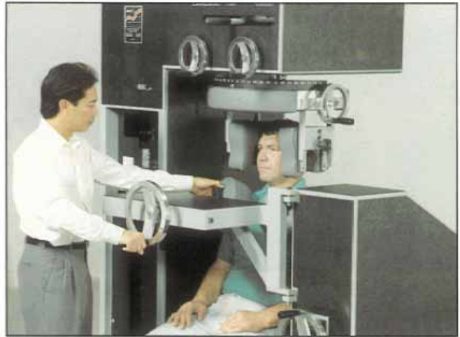
FIGURE 6-19 Unwanted movement of the torso is prevented by restraining the shoulders; adjustment of the shoulder pads being provided by the large wheel shown above.
